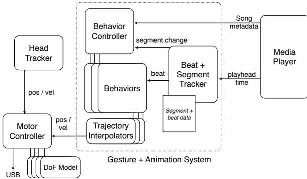
Fig. 5: Travis software diagram.
