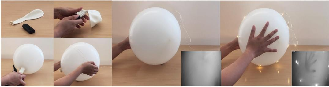
Fig. 15. Concept sketch of adding ShadowSense to a balloon. The balloon could become a touch-sensitive object, responding to touch by illuminating an LED strip.
