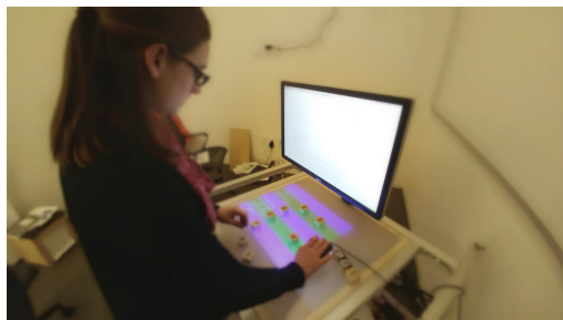
Fig 2. A user working collaboratively with an AI design agent using the presented digital-tangible sand table interface.
