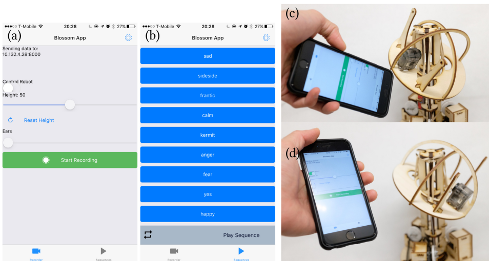
Fig. 11. Screenshots of the phone application for controlling the robot (a) and playing back gestures from within the application (b). The orientation of the phone is mapped to the orientation of the robot’s head (c and d).
